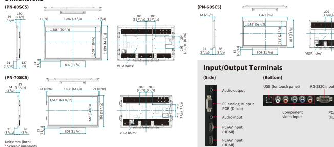
To use the VESA-standard mounting bracket, use M6 screws that are 8 to 10 mm plus the thickness of the bracket.
